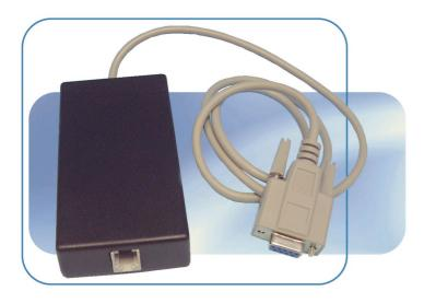
The HT12055 is a self-powered cash drawer interface packaged in a small in-line module complete with an industry standard RJ11 cash drawer connector.
